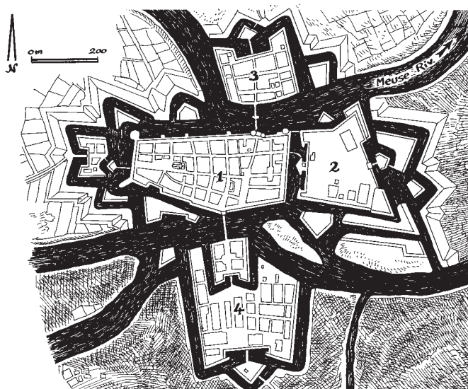
Fortifications of Mézières at the end of the seventeenth century. (1) Old medieval city; (2) military citadel built between 1590 and 1593; (3) northern suburb of Arches enclosed by hornwork; (4) southern suburb of Pont-de-Pierre enclosed by hornwork.
