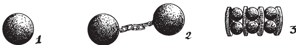
Ammunition. (1) Simple solid shot made of plain metal. (2) Two-chained shots. (3) Grapeshot (an early form of anti-personnel shrapnel).
