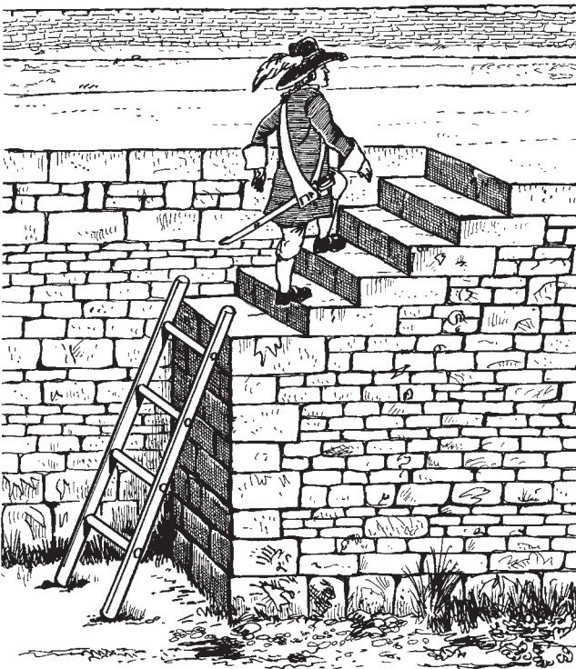
Place of arms. The re-entering place of arms is seen here from the gorge. (1) Ditch; (2) counterscarp; (3) pas-de-souris stair; (4) covered way; (5) traverse; (6) chicane passage; (7) sortie; (8) glacis.
