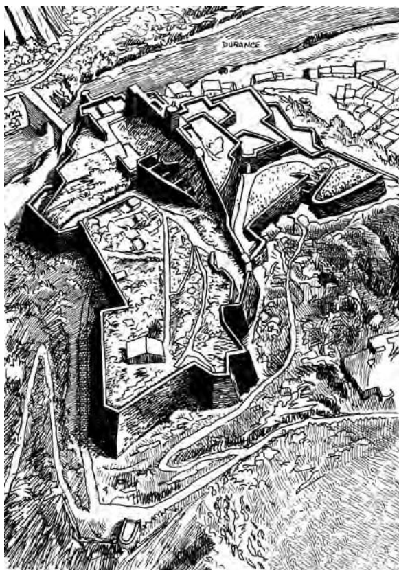
Citadel of Verdun by Jean Errard. Verdun, Toul and Metz were annexed to France under Henri II's reign in 1552. The Verdun citadel was built in 1640 after a design by Jean Errard. The shape of the bastion flanks illustrated very well Errard's typical style.
