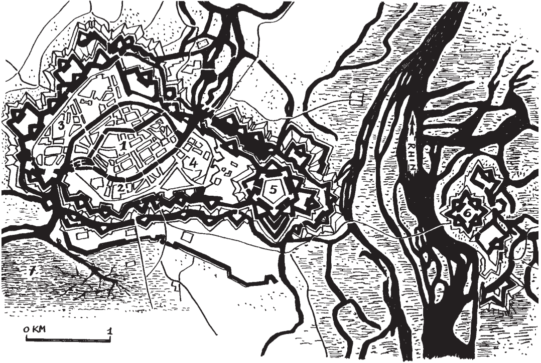
Strasbourg (1690). (1) Ancient city or Altstadt up to 1200; (2) medieval extension between 1228 and 1344; (3) second medieval extension from 1375 to 1390 on which Daniel Specklin built bastions (4) between 1577 and 1589; (5) Vauban's citadel; (6) Fort Kehl in Germany; (7) water defenses.
